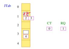
Thread 0 is running, thread 1 could run, threads 2 and 3 wait for the termination of 1, and thread 4 waits for the termination of 3.
