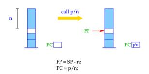
The instruction mark B allocates a new stack frame:
