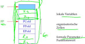
$FP \cong Frame \stackrel{1}{Pointer}$ ; points to the last organizational cell and is used for addressing the formal parameters and local variables.
