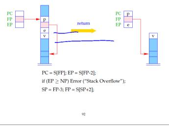
The instruction return pops the current stack frame. This means it restores the registers PC, EP and FP and returns the return value on top of the stack.
