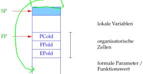
$FP \cong Frame$  Pointer; points to the last organizational cell and is used for addressing the formal parameters and local variables.
