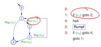
Bad: The loop body is jumped into.
