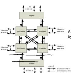
Processors in a NUMA system may be fully or partially connected.
