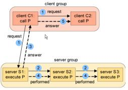
At any specific time, there is only one replica acting as master (primary replica); RPC requests are always propagated to the primary replica; at checkpoints the current state is propagated to the secondary replicas.
