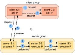
At any specific time, there is only one replica acting as master (primary replica); RPC requests are always propagated to the primary replica; at checkpoints the current state is propagated to the secondary replicas.
