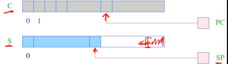
A virtual machine such as the JVM has the following structure:
