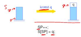
the instruction iconst q puts the int-constant q onto the stack
